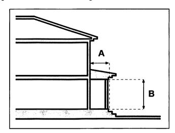
(4) Roofed front porches shall maintain a minimum width of at least 25% of the width of the *dwelling's* facade they are located on (illustrated as "A" below).
