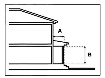
(4) Roofed front porches shall maintain a minimum width of at least 25% of the width of the *dwelling's* facade they are located on (illustrated as "A" below).
